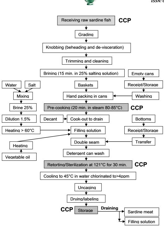
Figure 1: Flow sheet diagram of sardine canning
